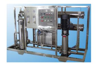
Reverse osmosis process utilizes a semi-permeable helix membrane to remove substances like dissolved solids, organic matter, colloidalmatterand bacteria in the water.
